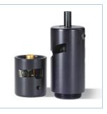
two pieces are threaded, so they can be assembled and stored as one unit, which protects the insides of the parts from damage. The jacket stripper is designed with a patented mandrel pin that supports the soft aluminum outer conductor and keeps it from being damaged during the jacket stripping operation.
